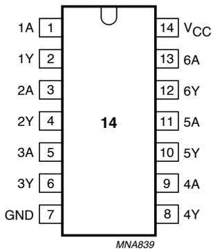
Fig.1 Pin configuration.
