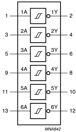
Fig.5 Functional diagram.
